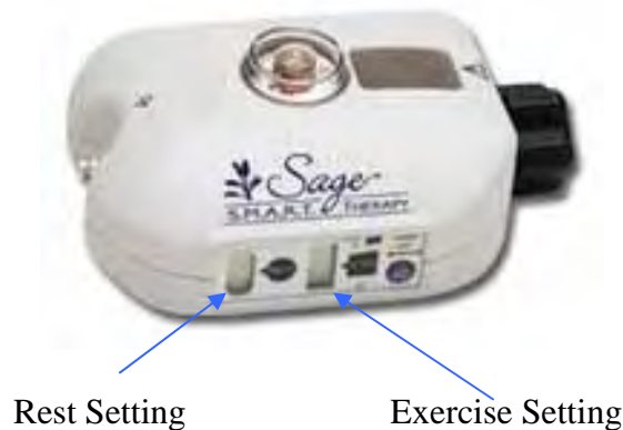
Figure 29 – Therapeutic oxygen delivery that automatically adjusts the oxygen setting during rest and exercise.
